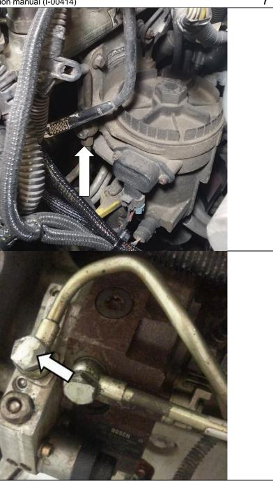
8. Pull the fuel bowl from the engine by removing the two bolts holding it in place using a 10mm Socket. Set these aside for re-install later.
