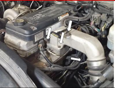
2. Place a pan or bucket below the fuel bowl and drain as much fuel out as possible by turning the drain valve. This will help reduce fuel spill when the fuel lines are disconnected.
