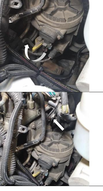
4. Disconnect the fuel heater and WIF sensor connectors.
