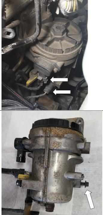
Remove bolt holding the return line to the back the of fuel bowl using a 10mm Socket. This fastener is not visible from the engine bay, and the bowl is shown removed for clarity. 6. Loosen and remove banjo bolts from both sides of the fuel bowl with a 17mm socket. Set these aside, as they will be used later for install.
